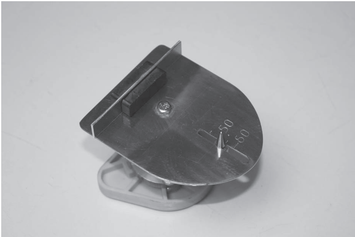
Figure 9. Special mounting table (or HIP-mount) with a longitudinal slot opening.
