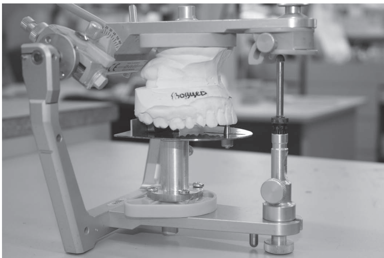
Figure 3. Model of the maxilla is placed in to articulator according to the HIP-plane.
